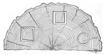
Fig. 63.—Shrinkage as affected by direction of annual rings; approximately twice as great tangentially as radially.
